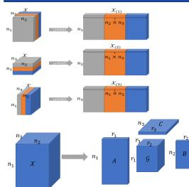
$\mathcal{X} \approx \mathcal{G} \times_1 A \times_2 B \times_3 C$  $x_{ijk} \approx \sum_{p=1}^{P} \sum_{q=1}^{Q} \sum_{r=1}^{R} g_{pqr} a_{ip} b_{jq} c_{kr}$  for  $i = 1, \dots, I, j = 1, \dots, J, k = 1, \dots, K.$
