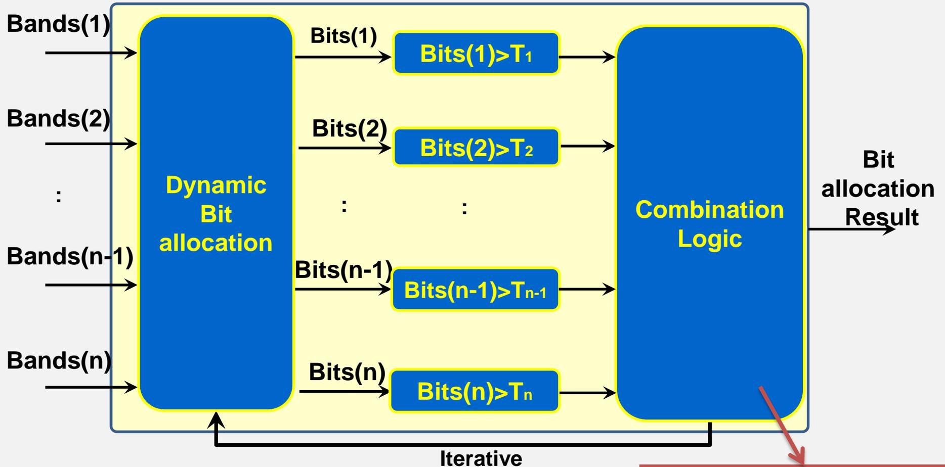
Bands with bits < Threshold identified and relocates bits to other bands
