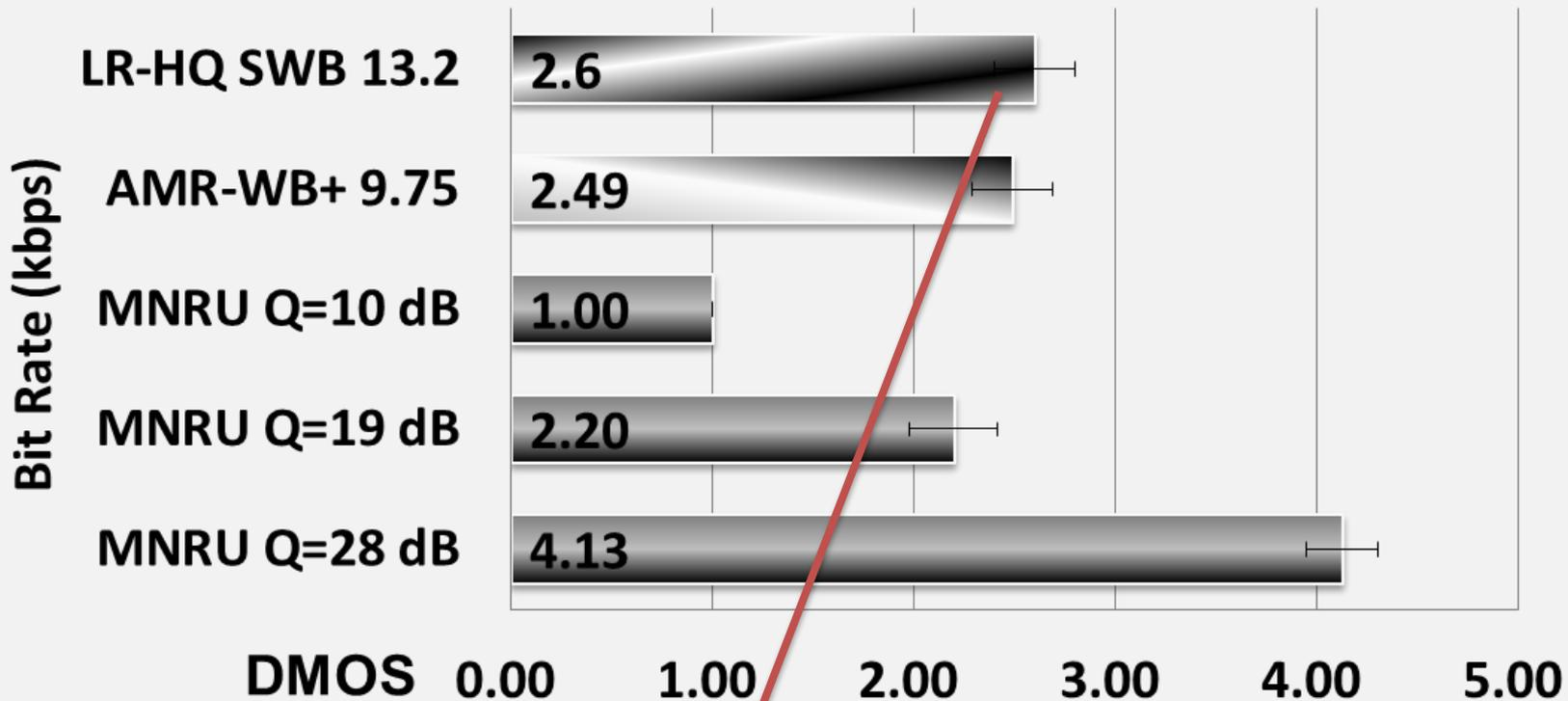
□ LR-HQ SWB Performance is equal or greater than AMR-WB+ whose algorithmic delay is longer than twice of EVS (32ms)
