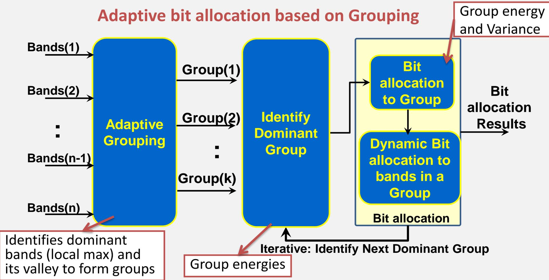
Bits allocated 1) **Adaptively grouping the bands** and 2) **By exploiting the relationship between the groups.**
