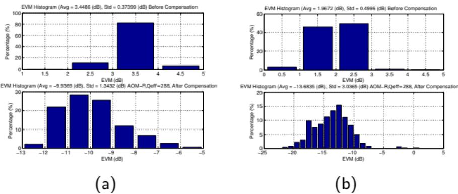
Figure: Effect of CFO Compensation on EVM: (a) OTA (b) OTC.
