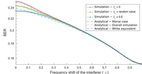
FIGURE 5 – BER abstraction, for  $P_{\text{Pol}} = P_{\text{interf}} = N_0$ .
