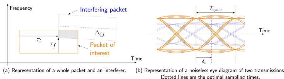
FIGURE 3 – Representation of a packet of interest (plain orange) and an interferer (dashed blue).
