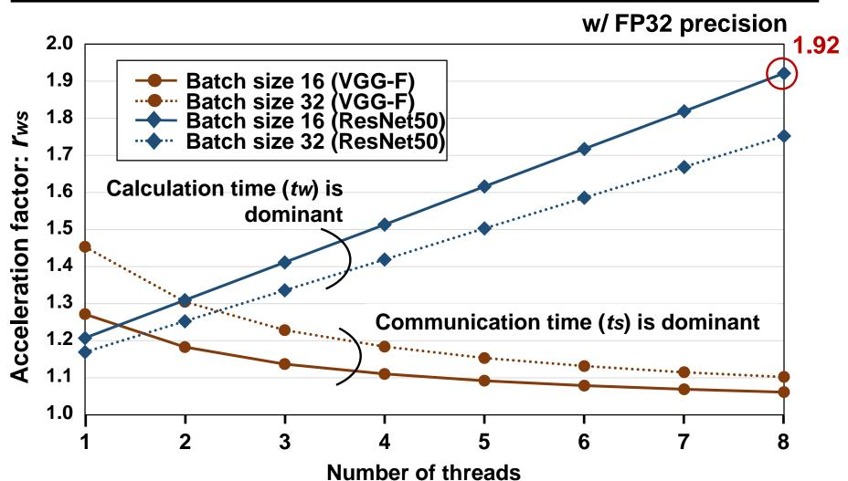
We calculated the ratio *rws* by measuring communication and calculation time. In ResNet50, rws reaches 1.92 when the number of threads is eight and the batch size is 16.
