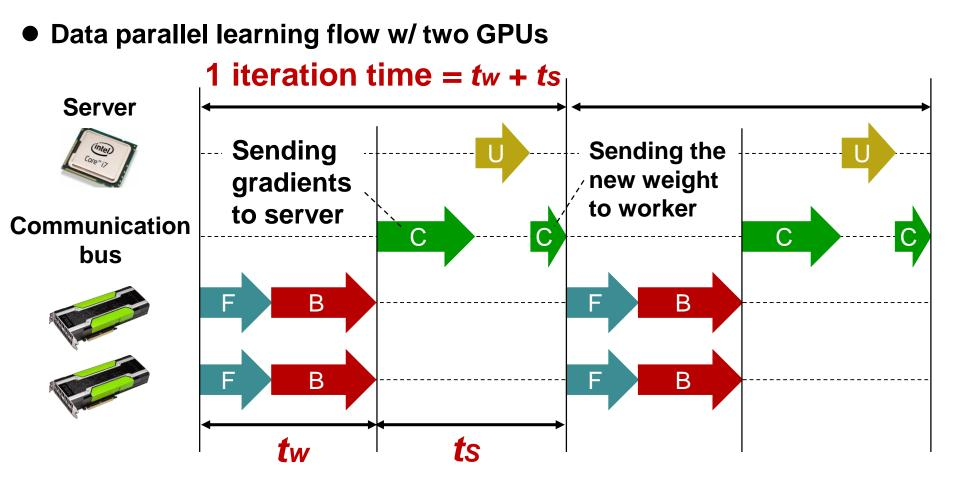
For worker, *ts* is the latency for next step. Particulary when the size of gradient is large, communication latency becomes bottleneck.
