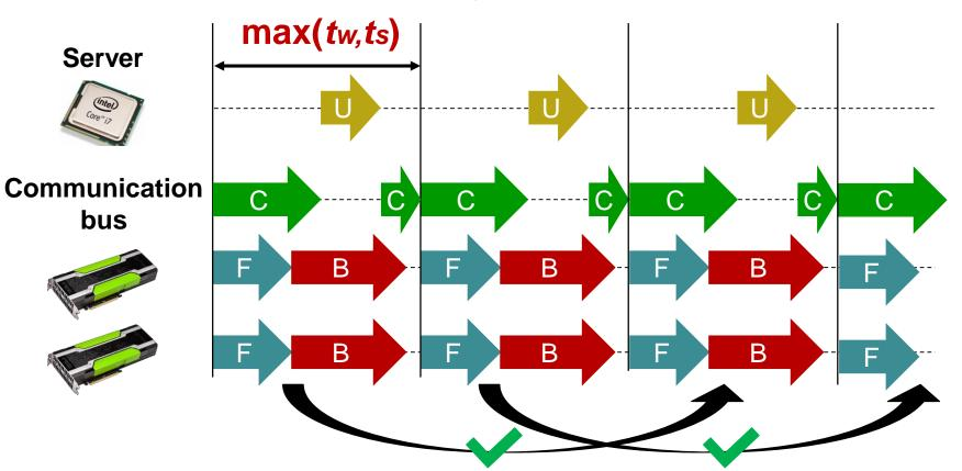
Gradient calculation reflects 2 steps earlier batch. The proposed method can eliminate the communication bottleneck.
