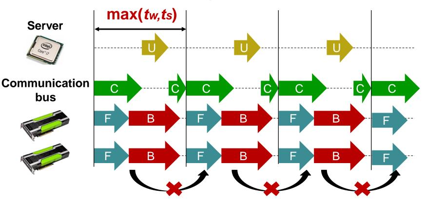
With proposed method, gradient calculation doesn't reflect the last batch update, and so we can overlap the parameter integration with the gradient calculation.
