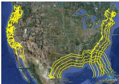
Figure: Shipborne radar exclusion zones in 3.5 GHz band (NTIA 2015).
