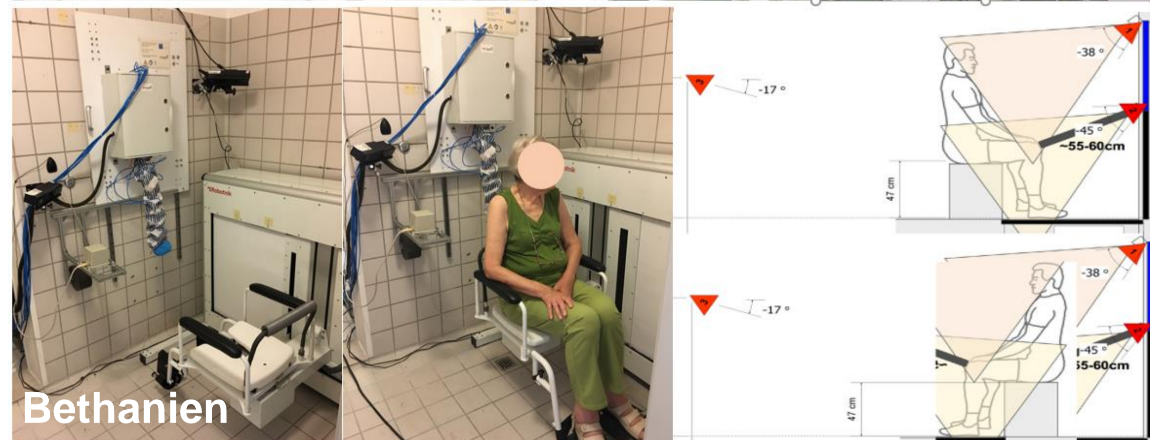
I-Support automatic bathing environment. Setup of the Kinect sensors as installed in the two validation sites: FSL (top) and Bethanien (bottom) hospitals.
