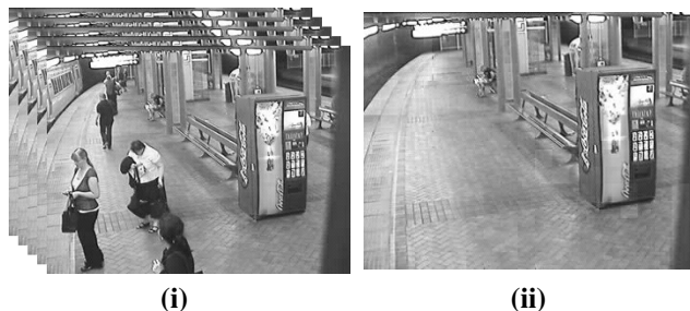
Fig. 1. Typical example of estimating the background from an cluttered image sequence: (i) input frames cluttered with foreground objects, where only parts of the background are visible; (ii) estimated background.
