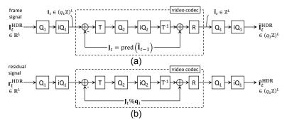
Fig. 1: (a) Block diagram for the video coding process with the effect of baseband signal quantization, and (b) equivalent diagram of (a). Block R is the rounding to the nearest integer operation, round(x).  $Q_i(x) \stackrel{\text{def}}{=} \text{round}(x/q_i)$ ,  $iQ_i(x) \stackrel{\text{def}}{=} q_i \cdot x$ , i = 1, 2 are quantization and dequantization, respectively. All operations are applied separately to each entry of x when x is a vector.
