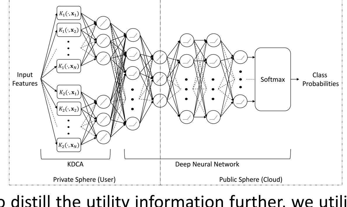
To distill the utility information further, we utilize a DNN with a narrow, *funneling layer*. The DNN processes multiple KDCA projections to form a **Compressive Hybrid**.
