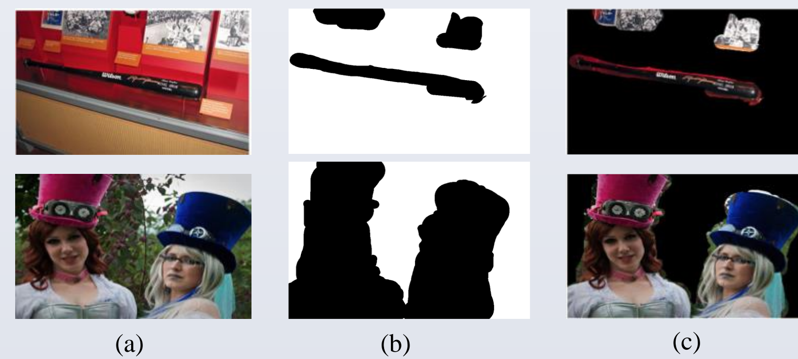
Fig. 2 Visual Objects Extraction: column (a) represents original images, (b) represent their corresponding event saliency maps while visual objects extracted via event saliency maps are shown in (c)
