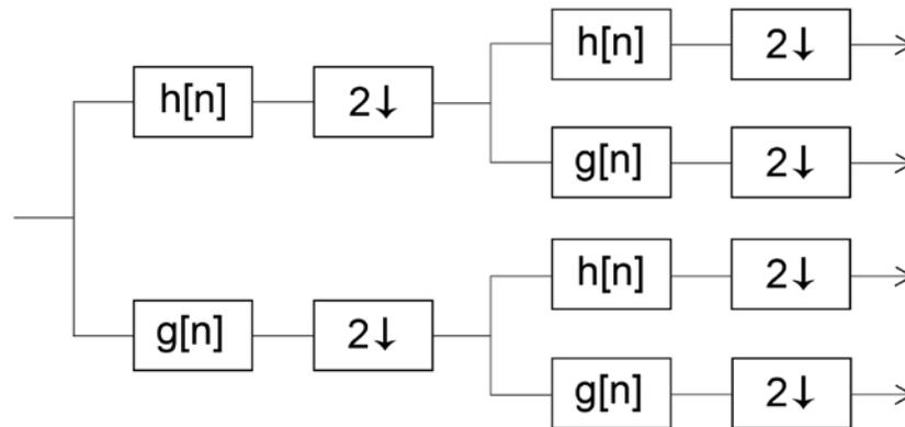
Fig-1 Wavelet Packet Decomposition
