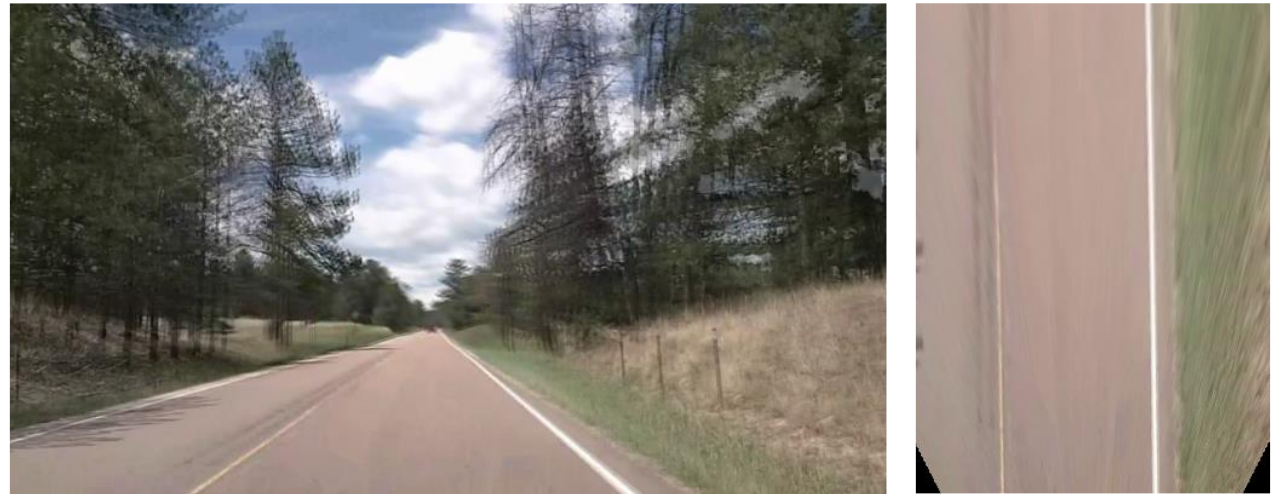
Fig 4. Input image and its remapped image using Inverse Perspective Mapping [4]
