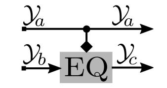
— EQ: Estimate and apply  $\mathcal{G}(\omega) = \mathcal{Y}_a(\omega)/\mathcal{Y}_b(\omega)$
