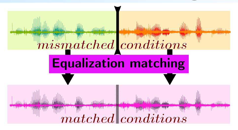
Equalization matching is the operation of matching the spectral balance of two signal segments.
