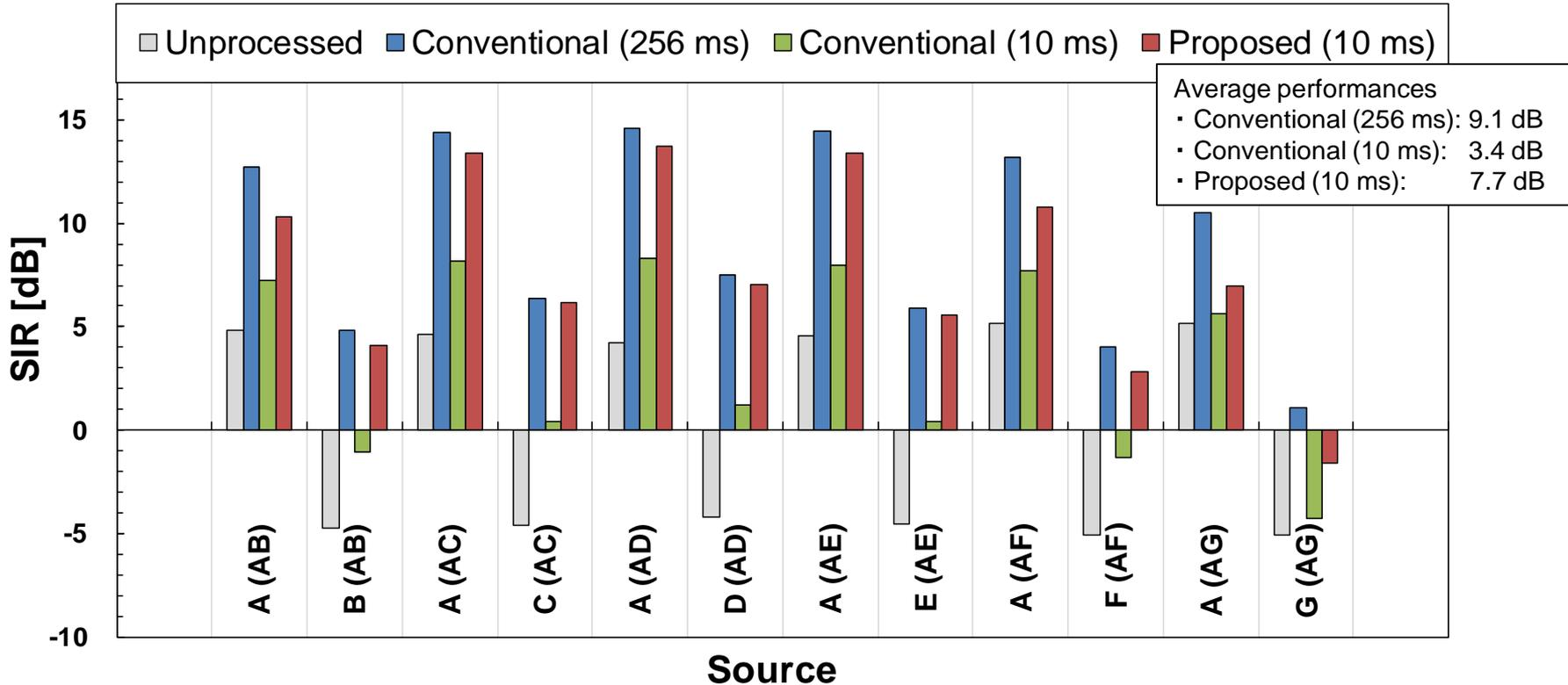
Separation performance of the proposed algorithm compared with that of the conventional algorithm with algorithmic delays of 256 ms and 10 ms
