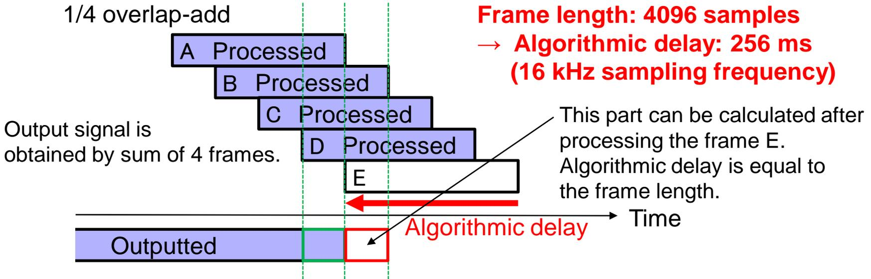
Image of the algorithmic delay for frequency-domain BSS
