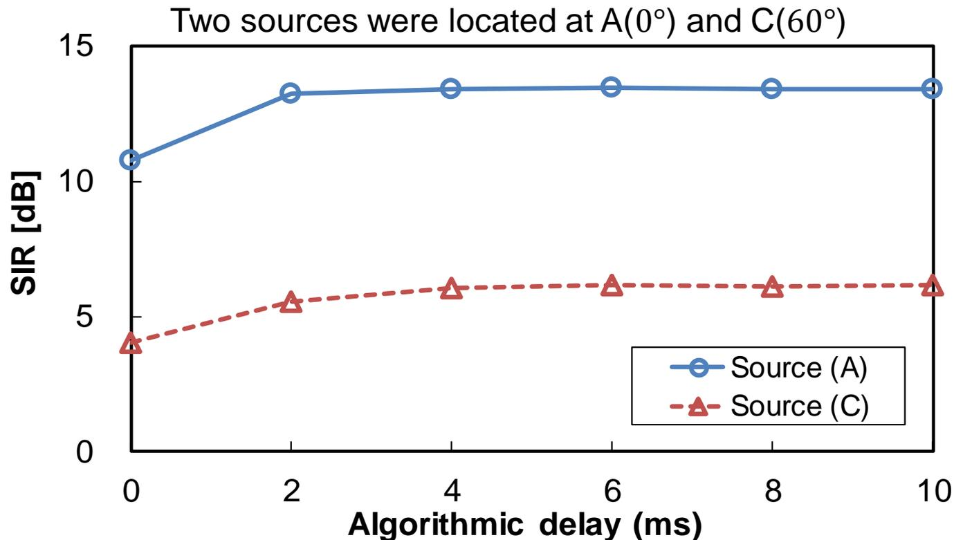
Resultant SIRs of the proposed algorithm for algorithmic delays from 0 to 10 ms. ( $N_d$  was set from 0 to 160 samples)
