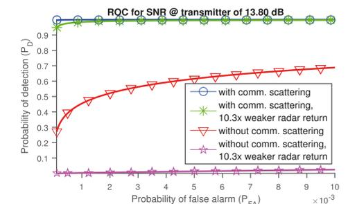
Fig 5. ROC curves showing that the detection capability decreases considerably when the communication signals scattered off the target are not exploited, especially when dealing with weak returns
