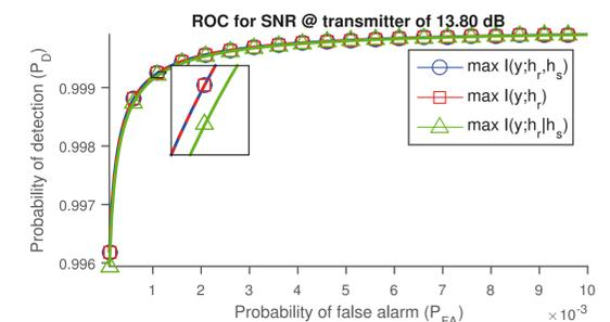
Fig 4. ROC curves showing that the radar waveforms that maximize  $I(\mathbf{y}; \mathbf{h}_r, \mathbf{h}_s)$  or  $I(\mathbf{y}; \mathbf{h}_r)$  provide better detection performance, despite  $\max I(\mathbf{y}; \mathbf{h}_r|\mathbf{h}_s) > \max I(\mathbf{y}; \mathbf{h}_r)$
