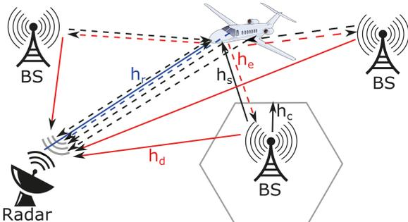
Fig 1. System model composed of the radar and communication base stations
