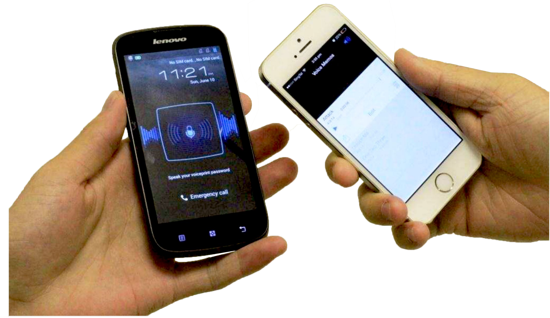
(Left) An example of audio replay attack [1]. The left phone (black color) is a smart phone with a voice-unlock function for user authentication; the right phone (white color) replays a pre-recorded speech sample to unlock the left phone.
