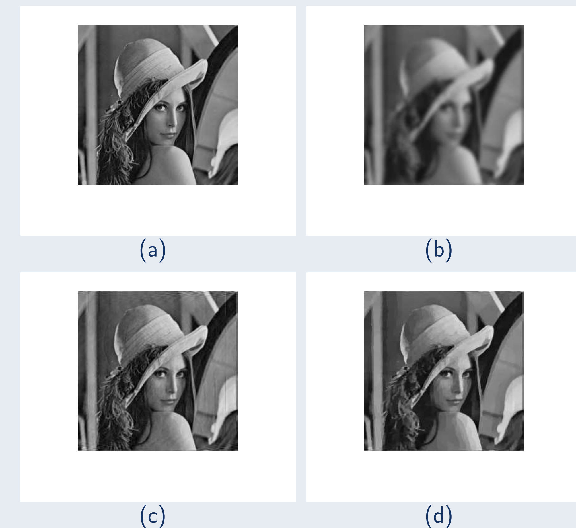
Figure: Deblurring results for Lena under Gaussian operator by using the two algorithms. (a) Original image; (b) Blurred image; (c) IRPAMC 16.0dB; (d) nonconvex ADMM 14.4dB.
