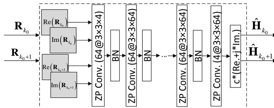
Fig. 2. Proposed CNN for joint channel estimation.
