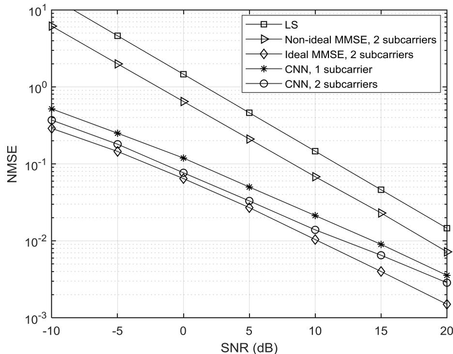
Fig. 3. NMSE versus transmit SNR for the proposed CNN based channel estimation and the existing methods.
