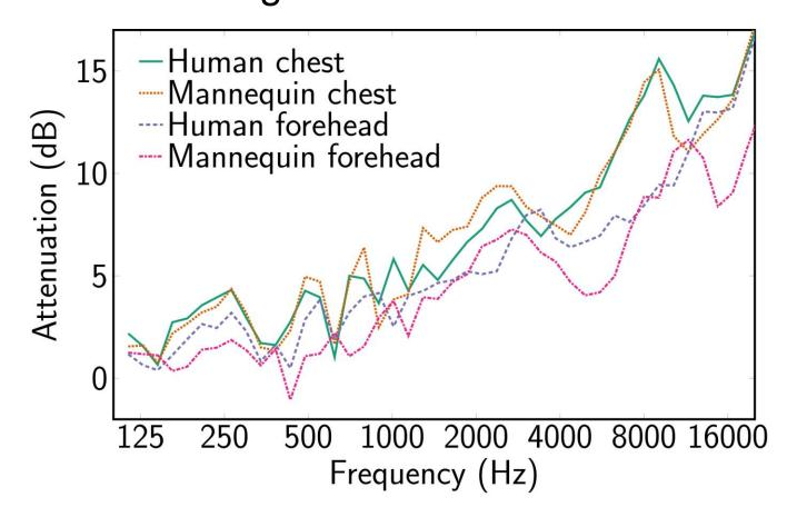
Average attenuation from sources on one side of the body to microphones on the opposite side of the body
