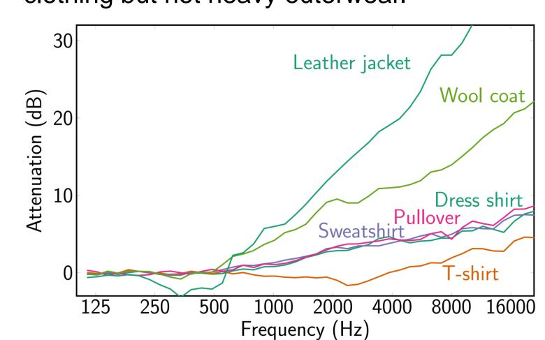
Average attenuation with clothing compared to uncovered microphones for sources on the same side of the body
