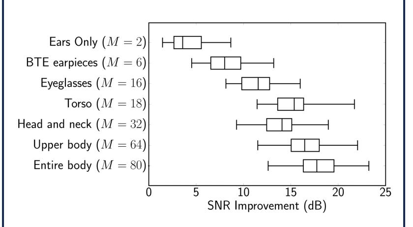
Average beamforming gain for an MVDR beamformer with 6 randomly selected speech sources
