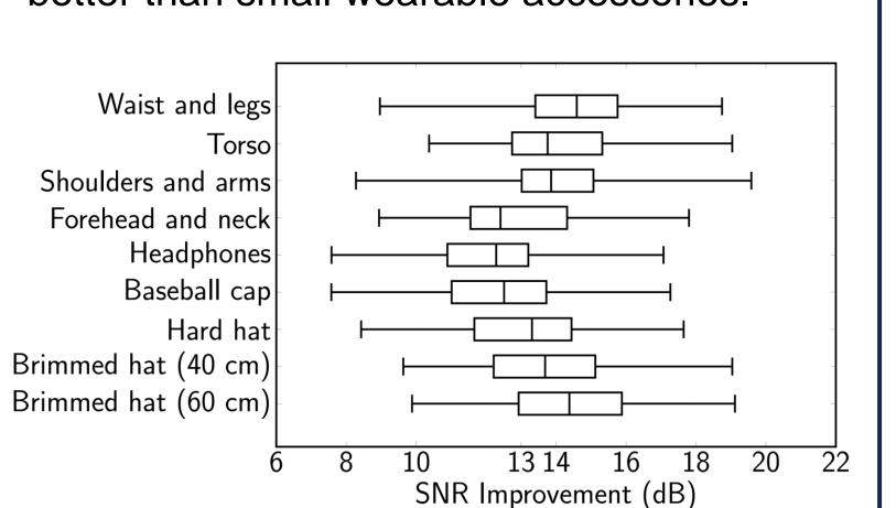
Average MVDR beamforming gain with 6 speech sources for arrays with different combinations of 18 microphones
