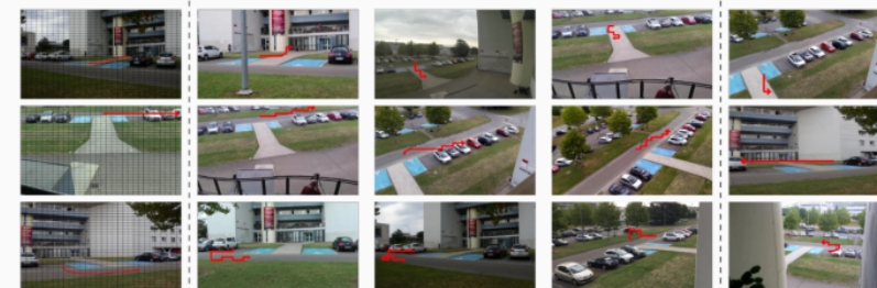
Best views ranking. 1st column: three trajectory queries are drawn in red, respectively for categories human, moto and car. 2nd to 4th columns: the top 3 views that offer a high visibility score are returned in descending order. 5th column: an overlapping view with a low rank.
