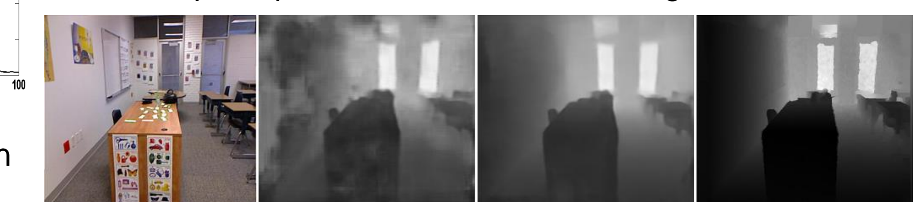
Figure: Visual results on NYU V2 dataset: First left - intensity image, Second left - result without using hourglass model, Third left - result with hourglass, Fourth column - ground truth
