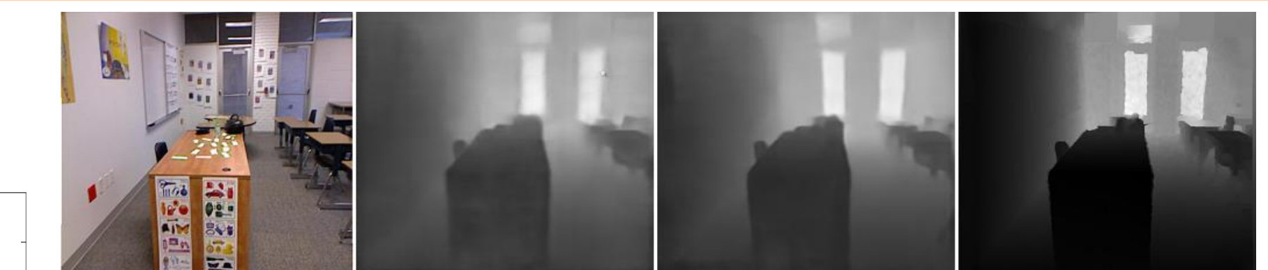
Figure: Visual results on NYU V2 dataset: First left - intensity image, Second left - result without perceptual loss, Third left - result with perceptual loss, Fourth column - ground truth.
