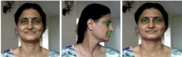
Figure 2: Result after recovery of feature tracking points. The features in the left part of the face are recovered, even after being
