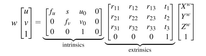
Perspective projection for HUD imaging, including linear transformations between different coordinate systems.
