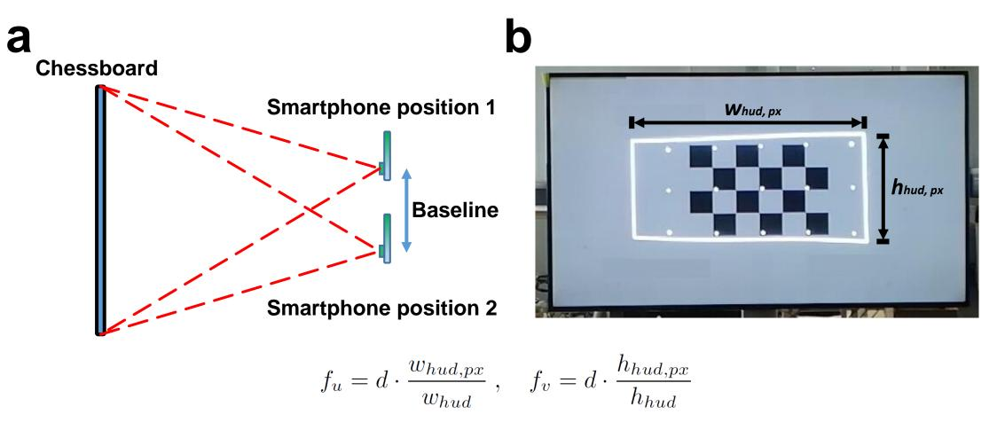
Assuming rectangular pixel (no skew) and the principal point falls onto the image center.
