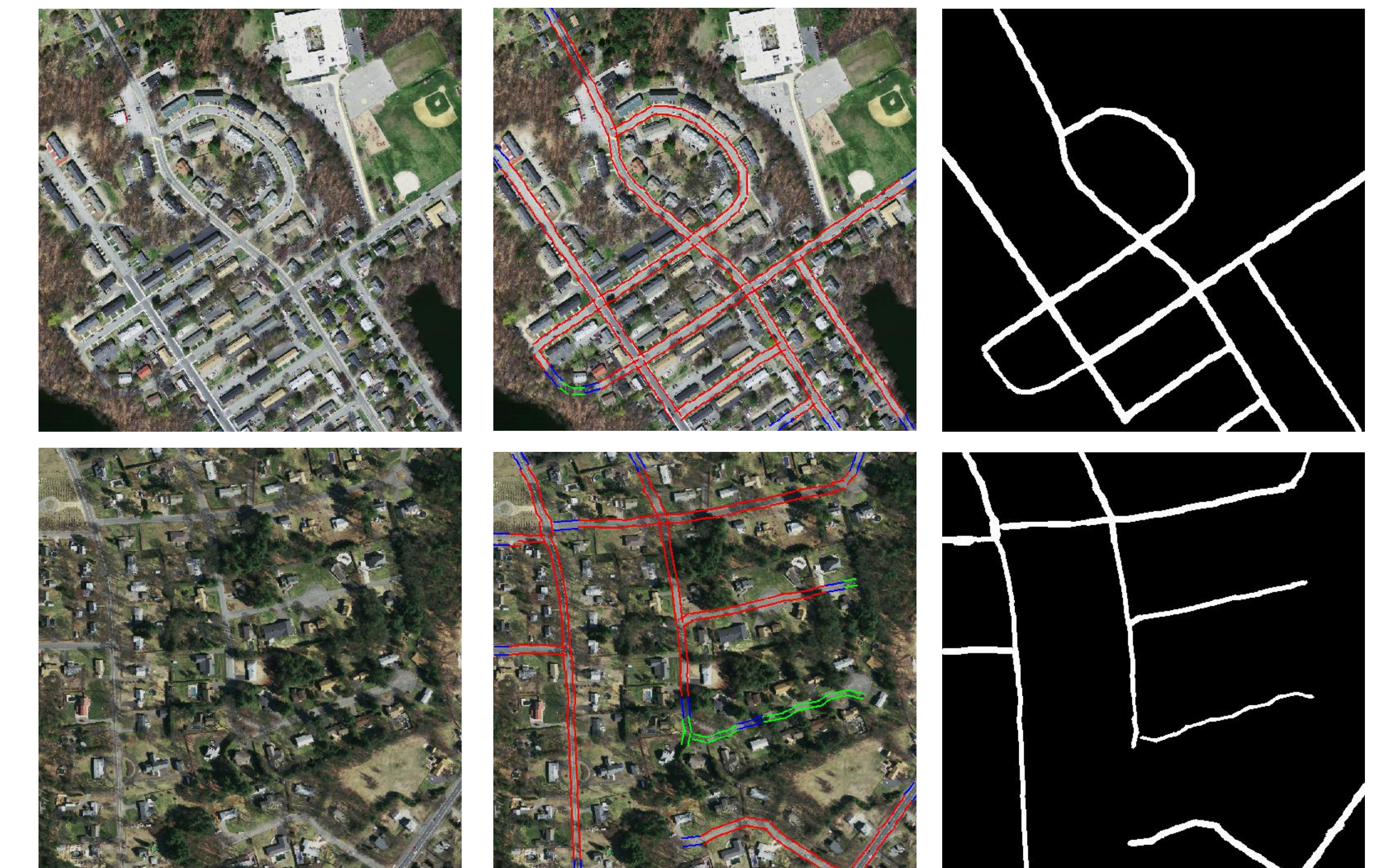
Fig 5. From left to right: original image, road extraction result, binary segmentation with extraction result. (Red: Closed tubes; Blue: Open tubes; Green: Tracking tubes)
