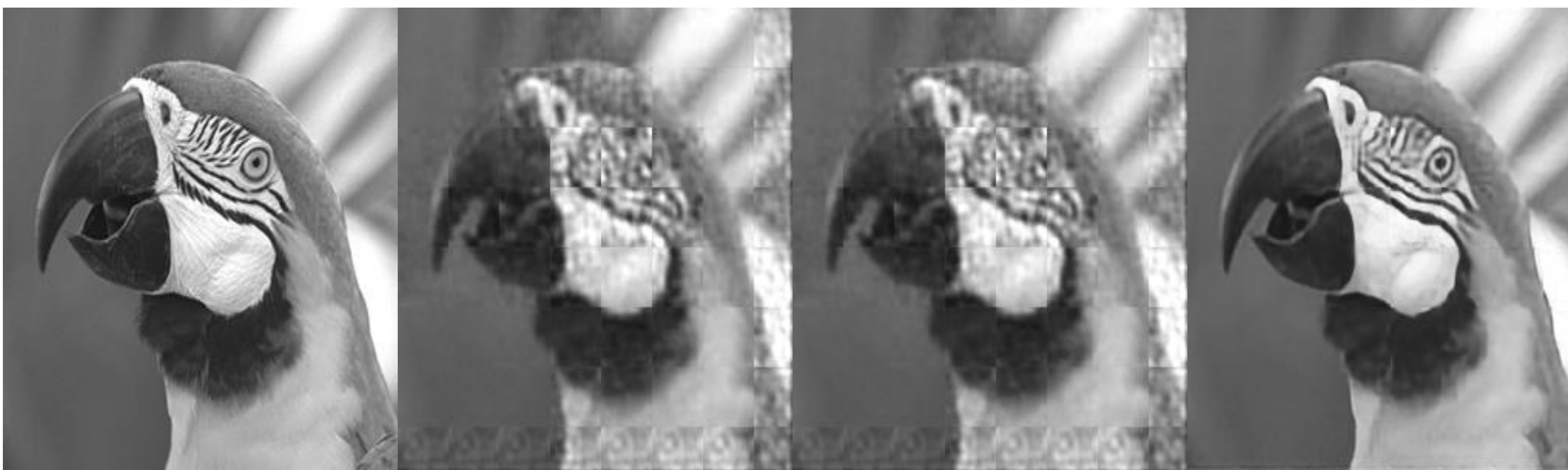
Ground truth 22.63dB/ 0.019s 23.94dB/0.057s 28.24dB/0.107s ReconNet DR 2 -Net Our MSRNet Fig.1 PSNR and time for recovering image "Parrots" at MR=10%
