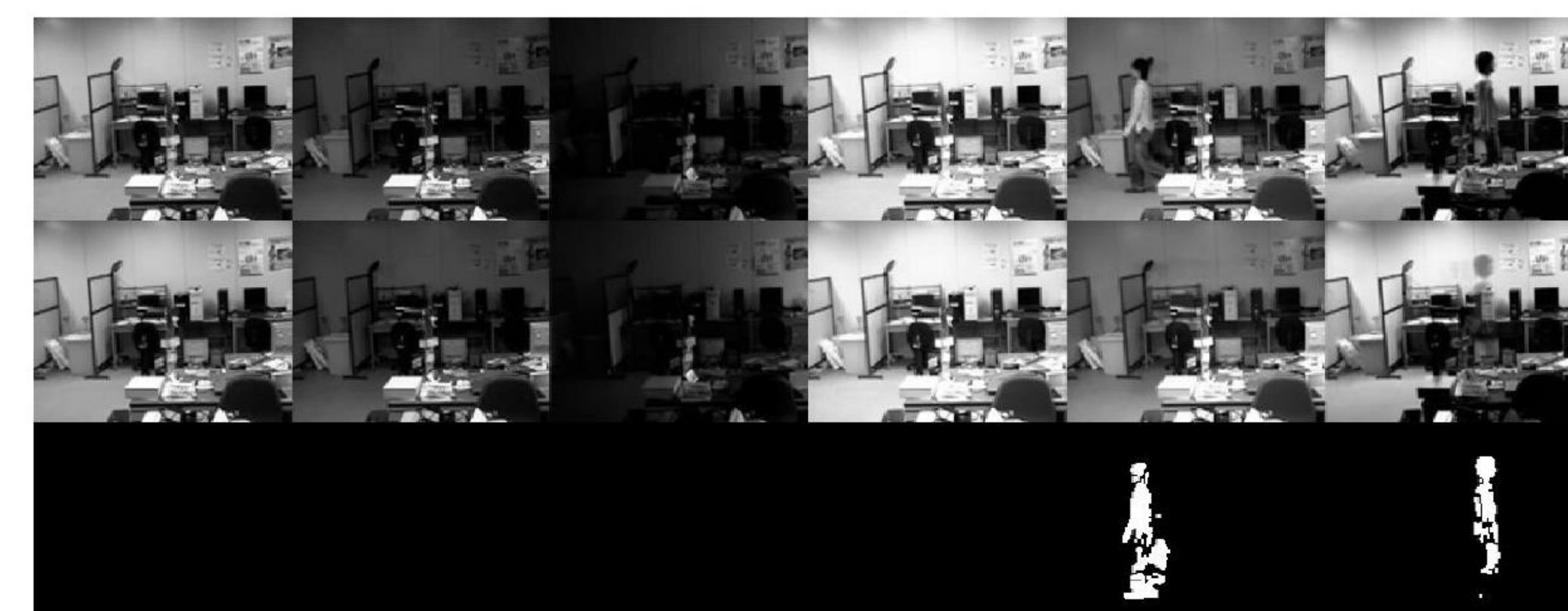
Fig 3. "Light switch" video from LIMU dataset, Top - Frames, Middle - Background estimation, Bottom - Foreground mask
