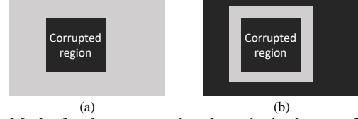
Fig. 2: Masks for the contextual and continuity losses. Gray and black colors denote 1 and 0, respectively. (a) Mask for the known part, \mathbf{M} , and (b) the boundary mask, \mathbf{M}_b
