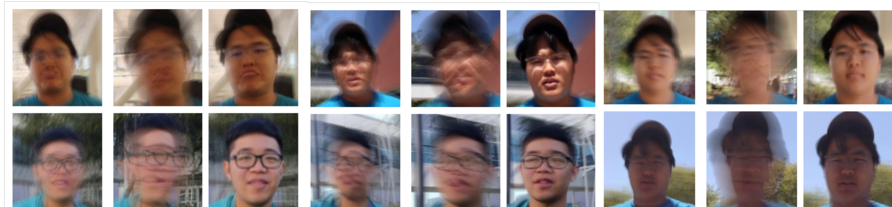
Face trajectory comparison between input (left), fused EIS (background only, middle), and Steadiface (right). Each frame is the average of consecutive 15 frames.
