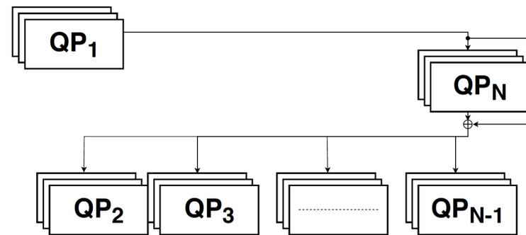
**CTU Depth Search:** Highest depth level in the lowest quality representation and the lowest depth level in the highest quality representation forms the CU depth level bounds for searching.
