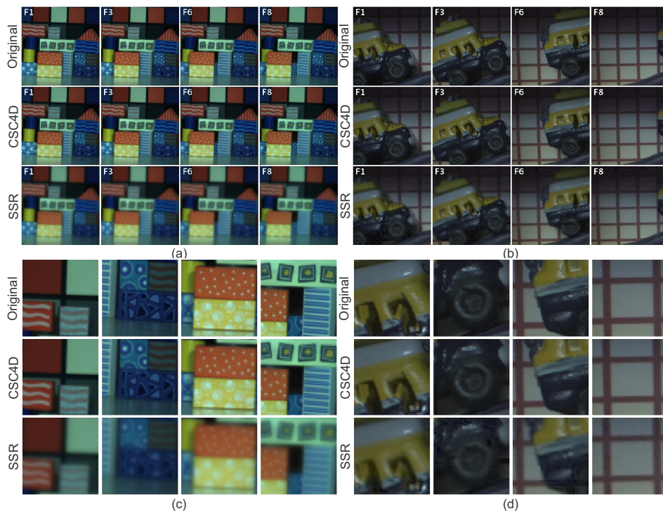
Figure 5: Example reconstructed frames with the CSC4D and SSR methods, for the datasets (a) Boxes and (b) Toy Truck, 256 \times 256 version, and some close-up details, (c) and (d)
