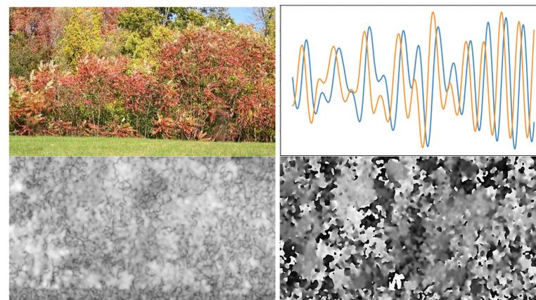
Fig. 3: Example dynamic motion sprite containing static background (upper left), horizontal motion signal (upper right), and the log amplitude and phase of the complex mode of horizontal motion (lower left and right).
