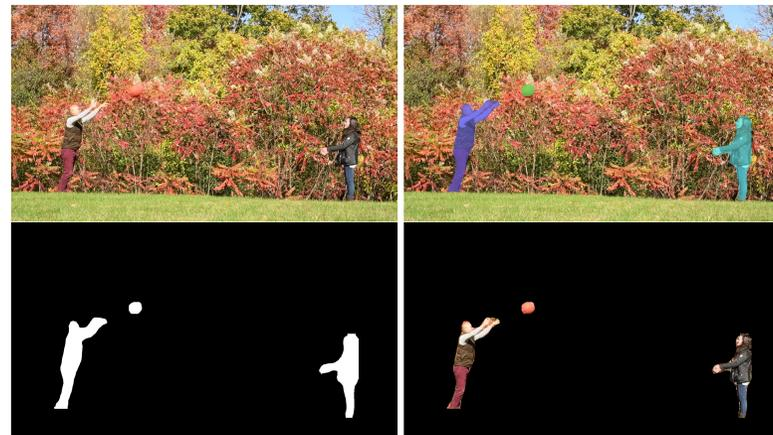
Fig. 2: Input frame (top left), instance level semantic segmentation masks generated by MaskRCNN (top right), with corresponding foreground mask (bottom left) and foreground content (bottom right). The bottom foreground and mask streams are compressed with AVC or HEVC and stored separately.
