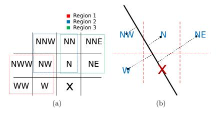
Figure 3: (a) Dotted boxes representing regions used for slope estimation; (b) Perpendicular distance of neighbors to the edge in EPI passing through the center of the current pixel.
