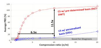
**Fig. 2**: Comparison of our proposed framework with conventional CS framework in term of CR.
