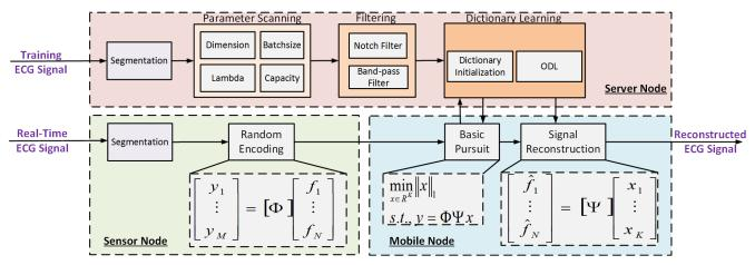
**Fig. 1**: Block diagram of the proposed framework. The parameter sweeping and dictionary training procedure are executed on servers. The reconstruction process is performed on mobile platform for providing timely feedback. The random encoding process using random Bernoulli matrix is embedded into the sensor node for effective data compression and energy saving.
