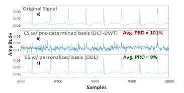
**Fig. 3**: Reconstruction result for a segment of ECG signal when CR=10. (a) Original ECG signal; (b) Reconstructed signal using pre-determined DCT-DWT joint basis; (c) Reconstructed signal using online trained dictionary.
