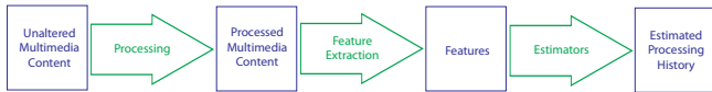
Fig. 1. Typical process that a multimedia signal may go through when considering forensics.
