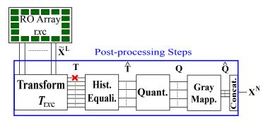
> Apply a transform  $T_{r \times c}(\cdot)$  to decorrelate  $\widetilde{X}^L / \widetilde{Y}^L$ ,
