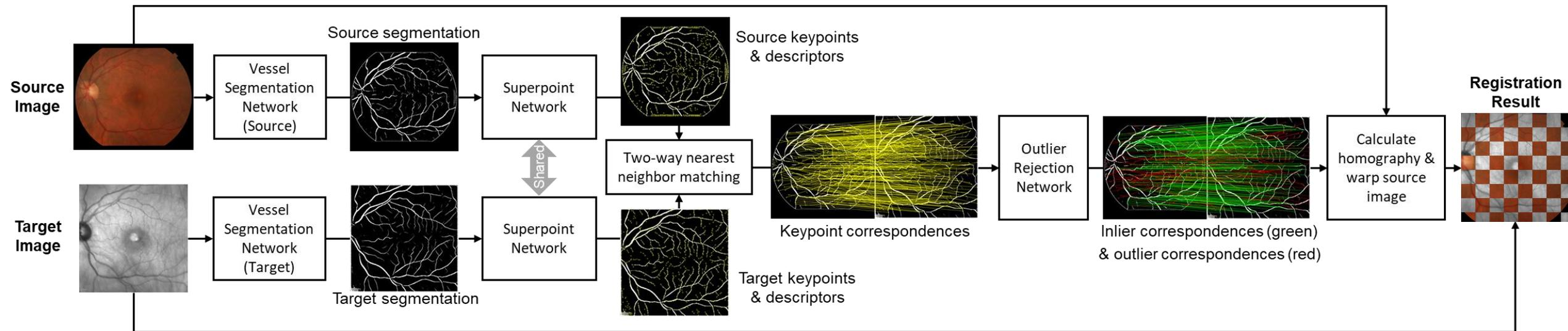
Proposed learning-based coarse alignment pipeline
