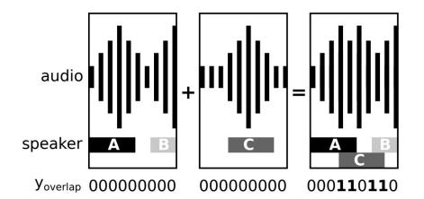
To increase the number of positive training samples for overlapped speech detection, artificial audio chunks are created by summing two random audio chunks
