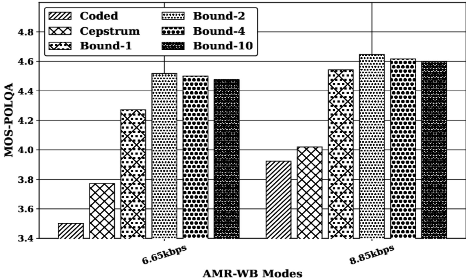
**Fig 1:** Average POLQA scores evaluating the oracle experiment at lowest 2 bitrates of AMR-WB (6.65kbps and 8.85kbps)
