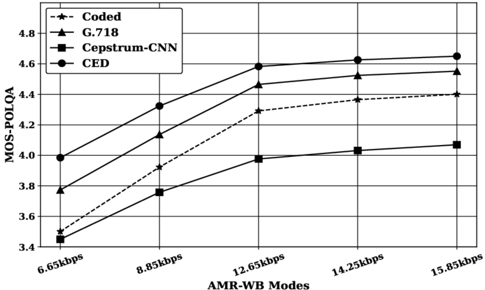
**Fig 4:** POLQA scores evaluating the performance of the Cepstrum-CNN, CED and G.718 using the NTT test set (lowest 5 modes of AMR-WB).
