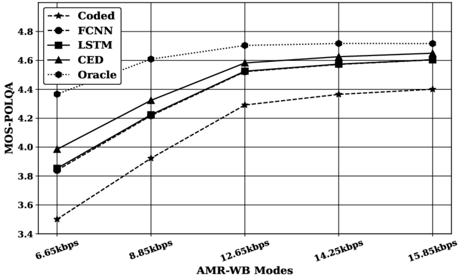
**Fig 3:** POLQA scores evaluating the performance of the FCNN, LSTM and CED architectures using the NTT test set (lowest 5 modes of AMR-WB).
