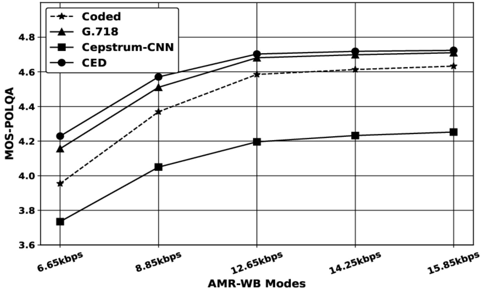
**Fig 7:** POLQA scores evaluating the performance of Cepstrum-CNN, CED and G.718 using the TIMIT test set (lowest 5 modes of AMR-WB).
