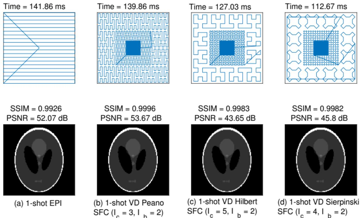
Figure: Performance comparison of single-shot VD SFC trajectories with EPI.
