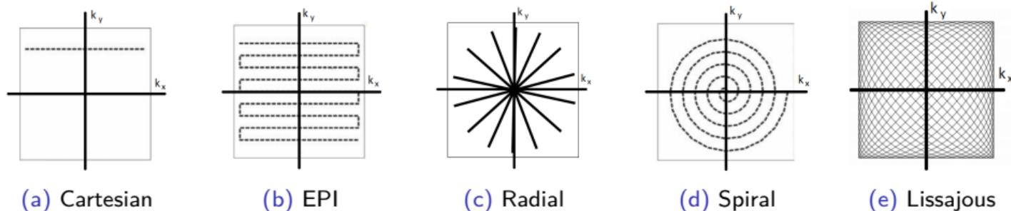
Figure: Various k-space trajectories in the literature.
