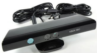
Microsoft Kinect (v1) sensor, featuring an RGB camera and a pair NIR-pattern emitter and NIR camera for depth sensing.
