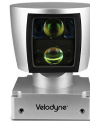
The Velodyne HDL-64E: A 64-channel LiDAR with 120m range, able to deliver up to 2.2 \times 10^6 points per second with <2cm accuracy.
