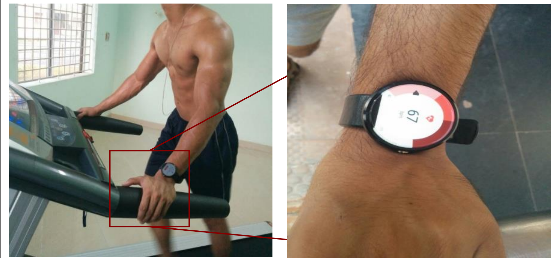
Real-time monitoring of heart rate (HR) from PPG during physical exercise on thread-mill using wrist band
