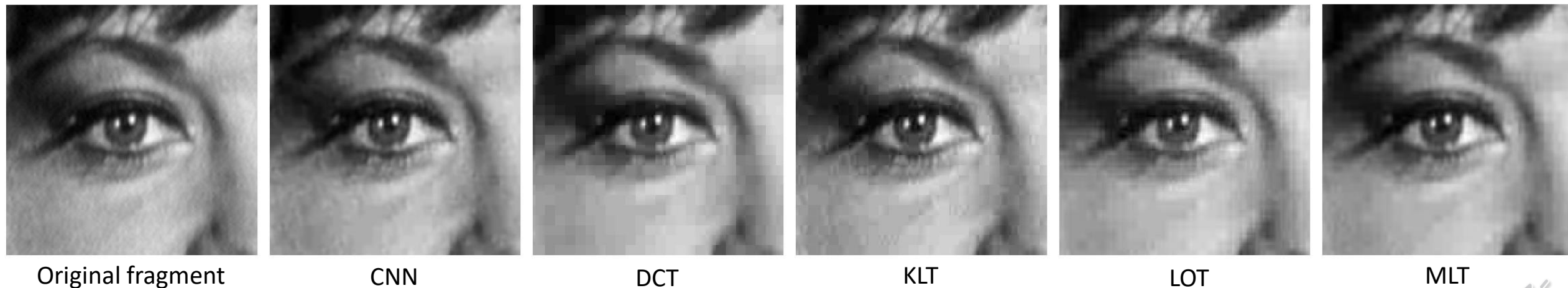
Fig. 8. Tiling effect reduction of CNN and other transforms based JPEG image compression scheme for 'zelda1024' image at 0.15 bpp .
