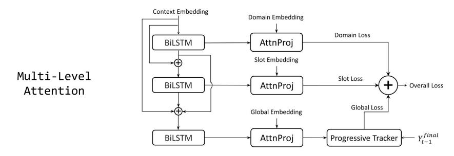
We adopt the attention mechanism on domain, slot, and global (combination of domains and slots) levels
