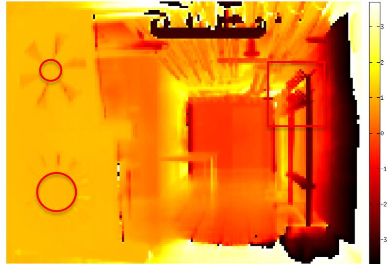
Depth image from a ZESS MultiCam (PMD PhotonICs 19k-S3)
