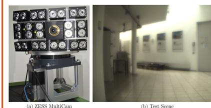
Figure 5: A ZESS MultiCam (a) was used to acquire real (LR) raw data. The observed scene was the hall of the ZESS building, shown in (b), with a depth range exceeding 16.5 m.
