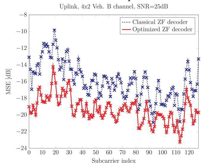
The optimal ZF decoder clearly outperforms the classical ZF decoder.
