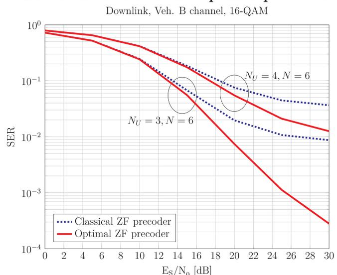
For a twice bigger number of BS antennas, the first order approximation of the distortion is cancelled and the SER does not saturate.
