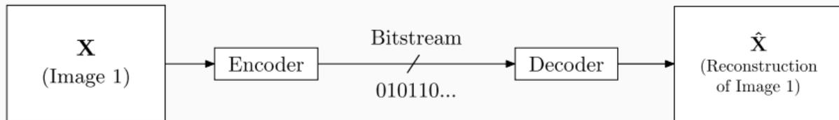
System model for point-to-point source coding.
