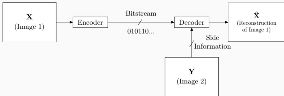
System model for source coding with decoder-only side information.
