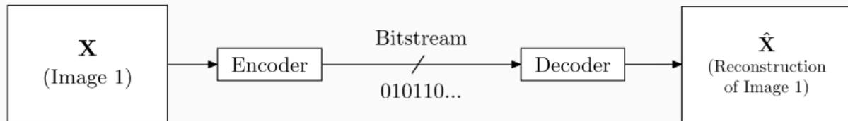
System model for point-to-point source coding.
