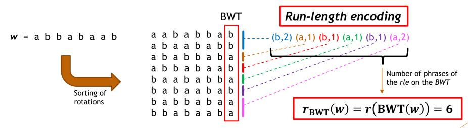
$\triangleright$  r(w): number phrases of the run-length encoding applied to w
