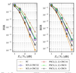
**Fig. 6**: Frame error rate (FER) and bit error rate (BER) performance comparison between CRC-aided SCL and PSCL decoding of  $\mathcal{P}(2048, 1024)$ . The code is optimized for  $E_b/N_0 = 2 \text{ dB}$ .
