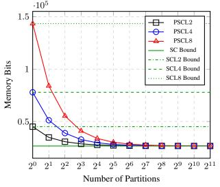
Fig. 5: Memory requirements for polar codes of length N = 2048. PSCLL (SCLL) denotes the PSCL (SCL) decoding algorithm with list size L.
